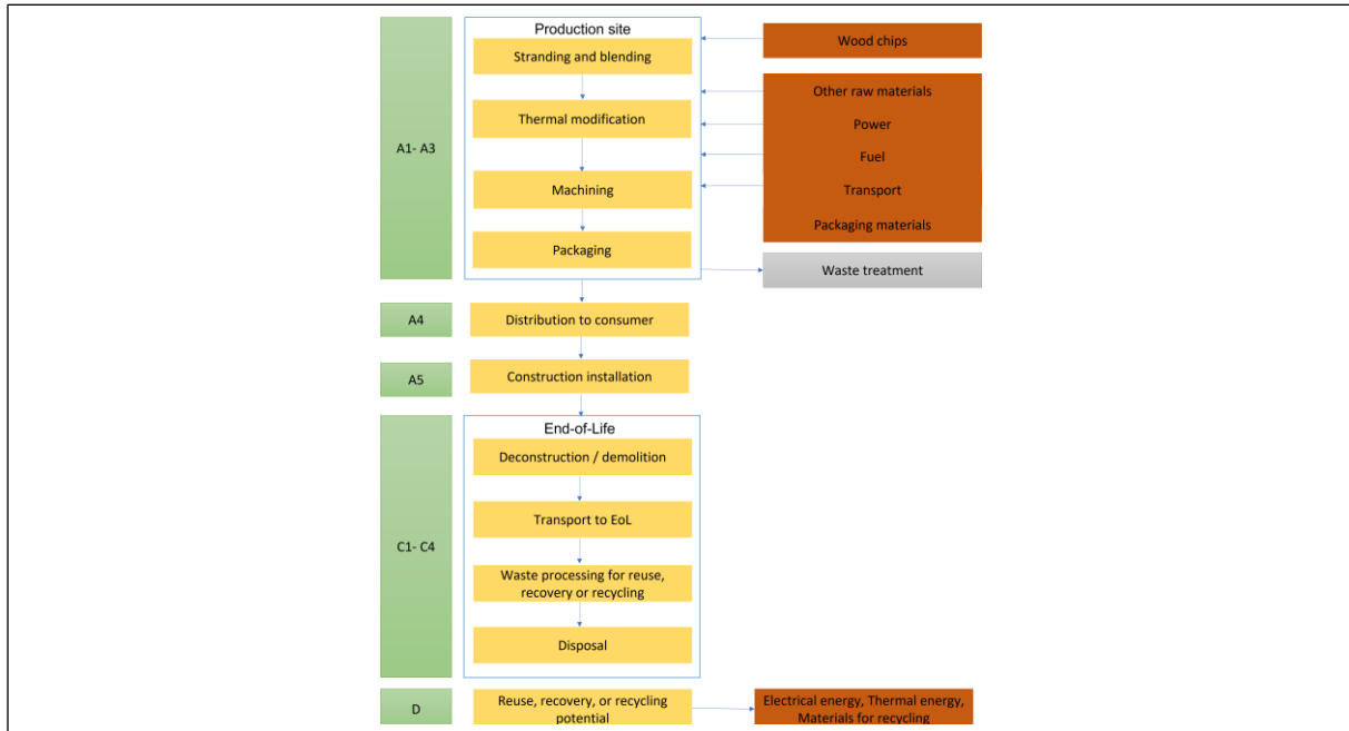
Figure 2: Process flow diagram showing the production and distribution of West Fraser MDF
